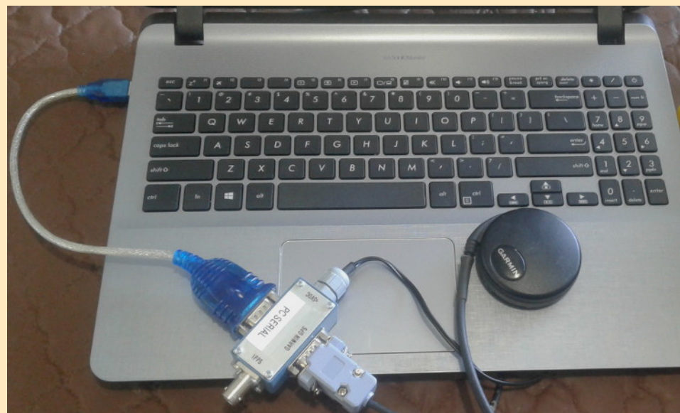
Updating firmware on a Garmin GPS 18x-LVC
