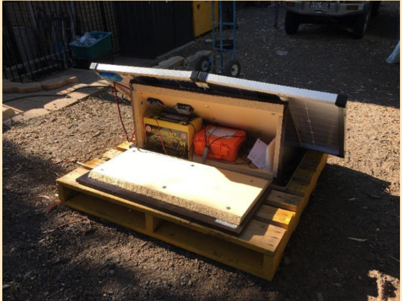
WAL1, a palletised portable seismic station made up of the usual suspects. 2 x 80W solar panels, a 12V 110AH lead acid battery, EchoPro recorder and Vodaphone network with an external antenna.
