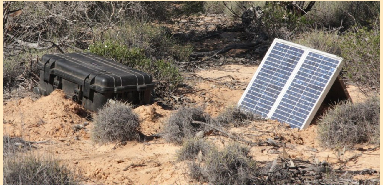
A typical deployment (seismometer is buried under the loose sand)
