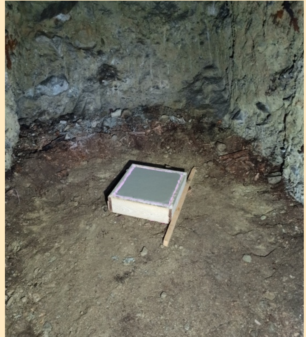
Figure 9: Instrument pier at the end of the OHERM vault
