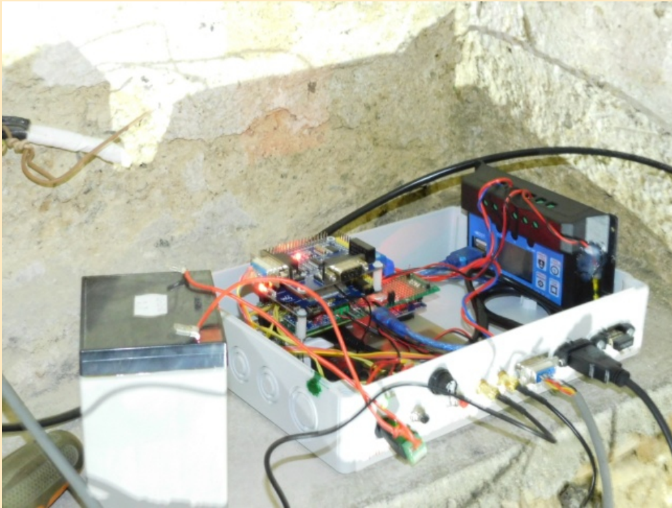
Figure 8: Testing of the autonomous RPiZero system controlling data acquisition
