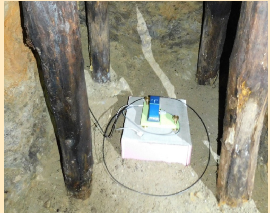
Figure 7: The LTS SOP5 sensor on the instrument pier at BREBA station
