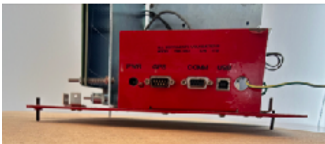
Figure 17 Showing the very thin base plate and coarse levelling screws
