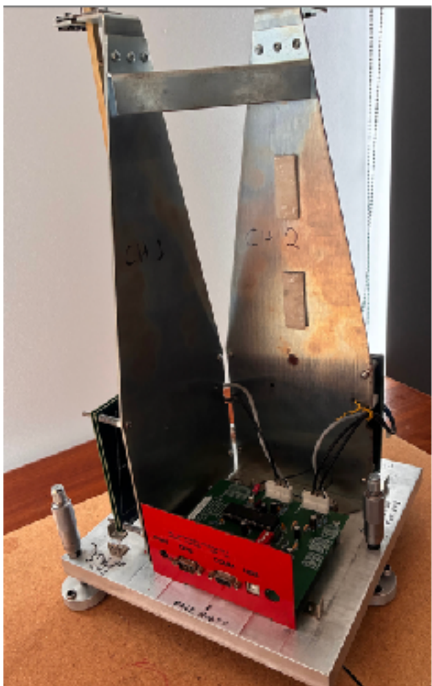
Figure 21 Showing 20 mm thick aluminium base. Three micrometer levelling screws each seated on a circular pad each pad with three pin support.
